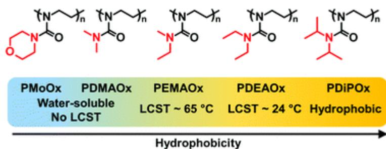
**Figure 6.** Structures of newly synthesized poly(2-amino-2-oxazoline)s. Reprinted from Publication P2.
