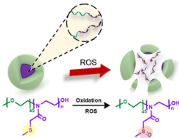
**Figure 8.** Structure of ROS-responsive block copolymer nanoparticles. Reprinted from Publication P4.
