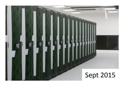
Rmax 0.08 PFLOPS 209x16x24x365= ~30 mil corehours/year Rmax 1.46 PFLOPS 1008x24x24x365= ~200 mil corehours/year
