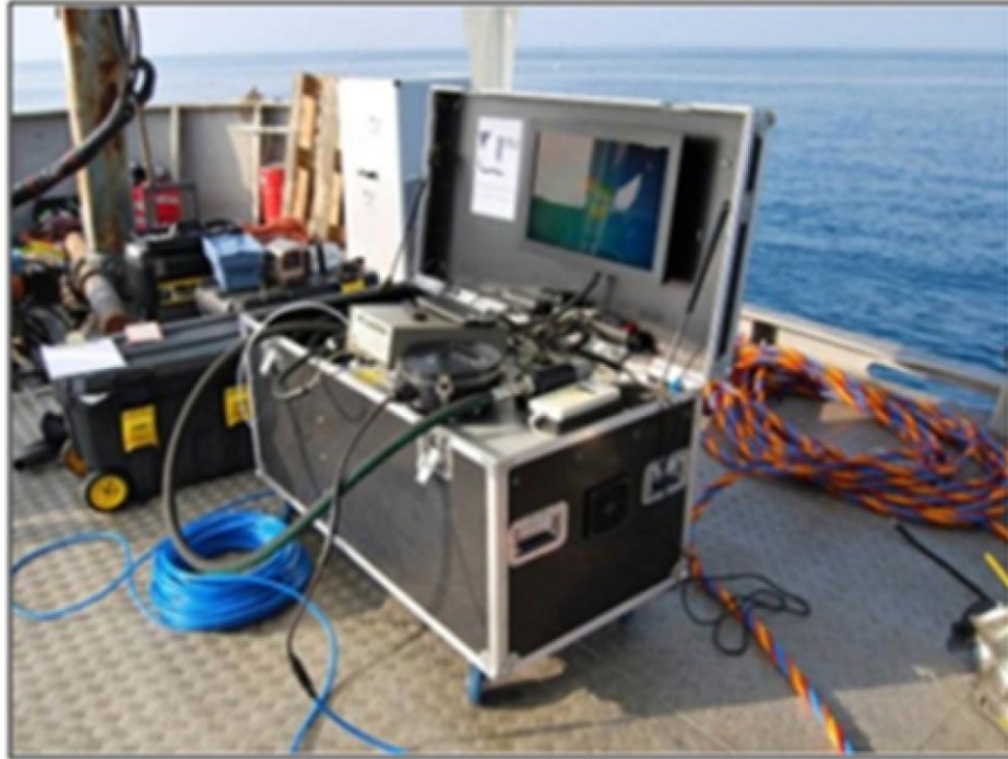
(a) Remote LIBS instrument on the research vessel
