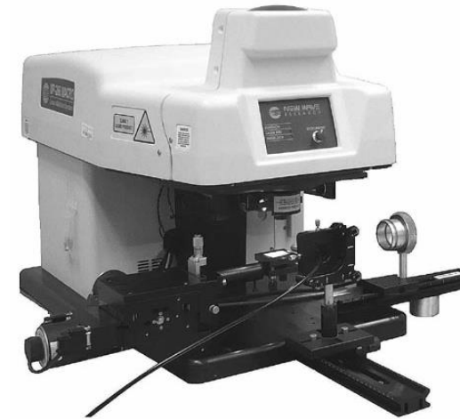
New Wave, UP 266 MACRO Nd:YAG laser @ 266 nm (4 th harmonic frequency) Second laser pulse Nd:YAG (Quantel Brilliant) @1064 nm
