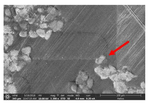
Combined DIC and fluorescence image of HeLa cells (left, acquired on TCS Leica SP8) cultivated on a dish with a grid shows the accumulation regions of Oregon Green labeled peptide. After chemical fixation and sample processing for FIB-SEM, the imprinted grid (middle SEM image) was used to identify the particular cell and localize the target site (red arrow). Subsequent 3D FIB-SEM acquisition reveals the targeted volume ultrastructure (single slice image on the right).
