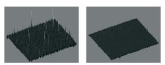
Dark image comparison with the measured distribution of "hot blinking" pixels at 5°C of the image sensor. The left image gives a 3D view with the sophisticated "blinker filter" algorithm off and the right image shows the result with the filter switched on.
