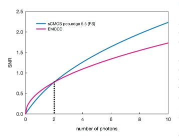
The graph shows the signal-to-noise (SNR) curves of a typical emCCD camera (gain = 1000) and a pco.edge 5.5 camera vs. number of photons.
