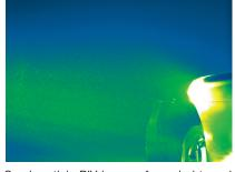
Seed particle PIV image of an wind tunnel experiment (false color rendering) to improve the aerodynamics of a racing car, courtesy of ILA GmbH & Toyota Motorsport, Germany
