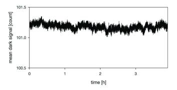
Mean dark signal drift measurement of a pco.edge camera stabilized at +5 °C over a 4 hour period record at 100 frames/s (1 count = 0.5 electron).
