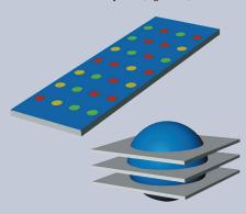
The GenePix Professional 4200A optical path is designed specifically for microarrays. Confocal optics do not benefit microarray imaging, because the primary source of background is in the same plane of focus as the sample (left). Confocal imaging is primarily beneficial for rejecting out-of-plane background when scanning a thick sample (right).
