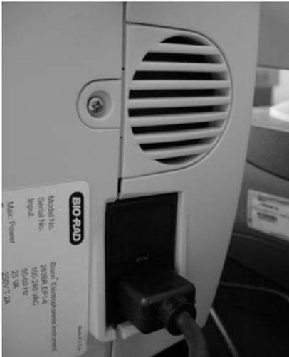
Figure 1.5.2a. Power connection for electrophoresis station.
