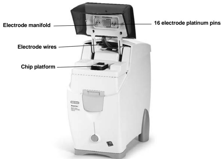
Figure. 1.3.1b. The Experion Electrophoresis station with lid open.
