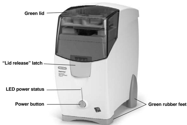
Figure. 1.3.1a. The Experion Automated Electrophoresis station.
