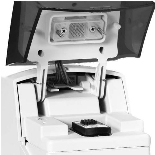
**Figure. 2.6b. Proper chip placement in the electrophoresis station.**
