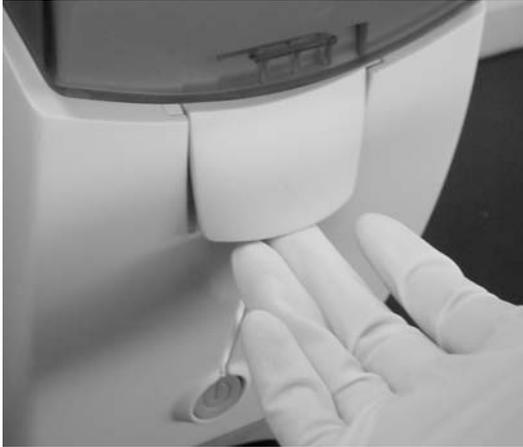
**Figure. 2.6a. Opening the electrophoresis station.**
