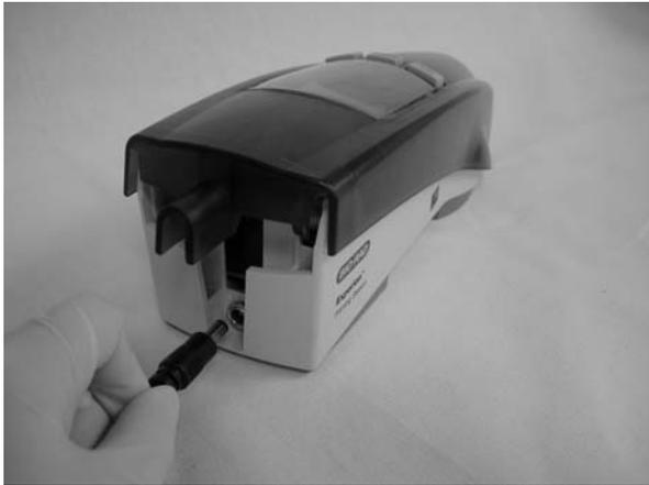
**Figure. 1.5.2c. Power connection on the priming station.**
