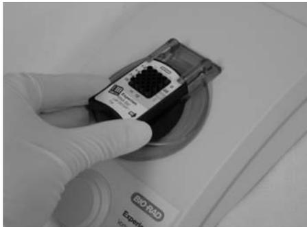
**Figure. 2.5.** Inserting a chip into the vortex station.
