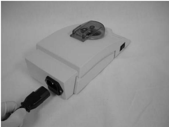
**Figure. 1.5.2d. Power connection on the vortex station.**
