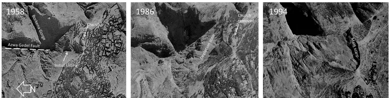
Fig. 10 Subsets of aerial photos of the Doro Mezleya locality provided by the Ethiopian Mapping Agency showing that the sliding occurred there in several phases. The major sliding took place between 1986 and 1994
