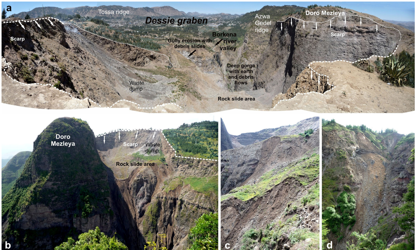
Fig. 9 Doro Mezleya landslide area: a view from the upper southern edge of the scarp towards the Dessie graben with the Borkena river valley, b view of the whole landslide area from the Azwa Gedel ridge pathway, c small reactivation in the central part of the landslide area partially influenced by quarrying activities, d rock fall in the erosion gully adjoining with landslide area to the north (photo Z. Vařilová)
