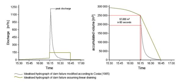
Fig. 5. Approximate hydrograph of the event (based on the recorded time sequence of the dam failure).
