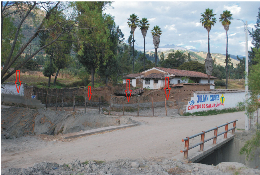
Fig. 11 The flood mark on Station 0.885 km is indicated by grey mud on the partly destroyed adobe wall. The photograph was taken by the authors during fieldwork in 2010
