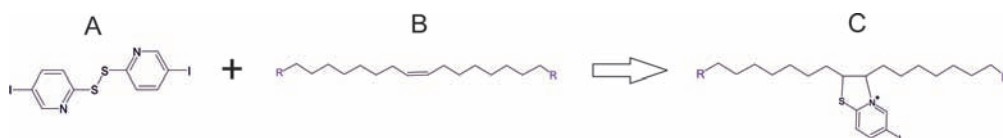
Fig. 1 Scheme of derivatization reaction: (A) bis-(5-iodo-[2]pyridyl)-disulfide, (B) lipid with double bond, and (C) derivatized lipid, the reaction product.
