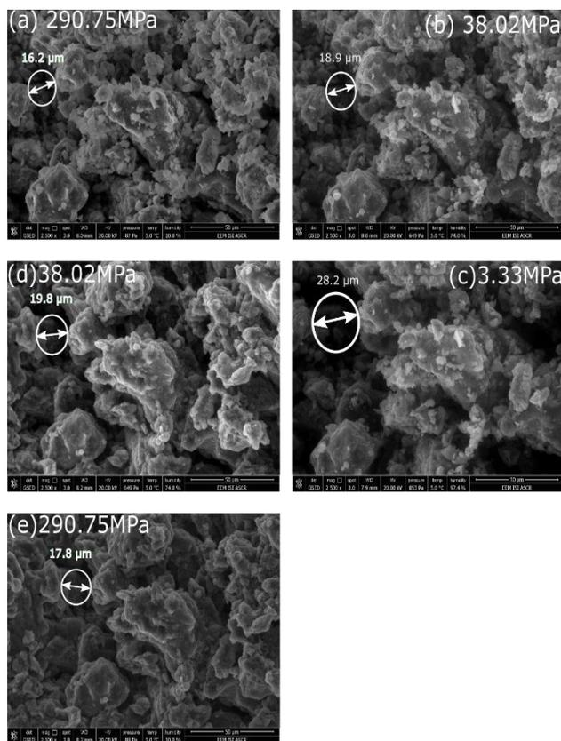
Figure 6. Selected ESEM micrographs of compacted bentonite with a dry density of 1.27 Mg/m<sup>3</sup> under the wetting-drying path. (a),(b),(c)-wetting path; (c),(d),(e)-drying path.
