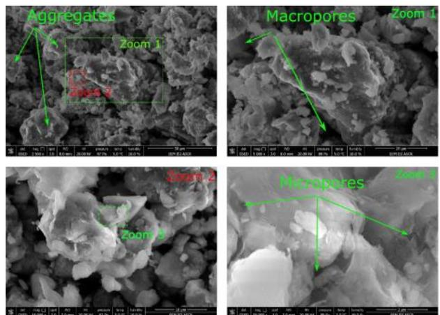
Figure 5. ESEM micrographs of compacted bentonite with a dry density of 1.27 Mg/m<sup>3</sup> at different magnifications.
