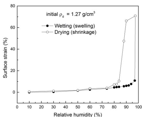
Figure.8 Surface strain versus relative humidity for compacted bentonite along wetting and drying path, sample with initial dry density of 1.27
