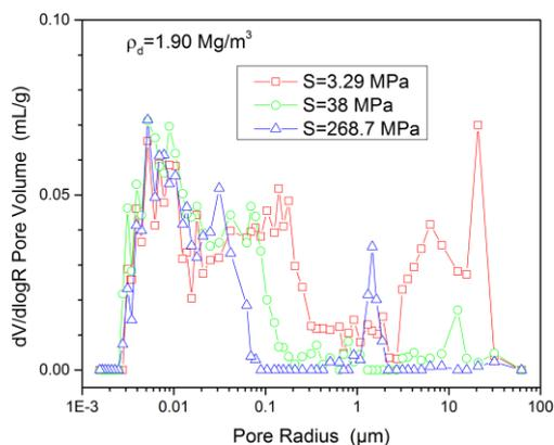
Figure 4. Pore density function curves of initial dry density of 1.90 Mg/m<sup>3</sup> at three suction level
