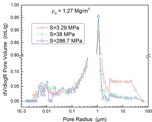
Fig 3. Pore density function curves of initial dry density of 1.27 Mg/m<sup>3</sup> at three suction level
