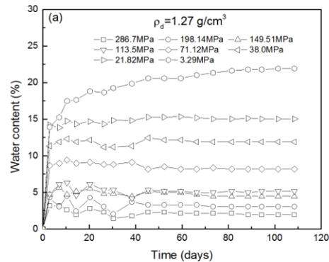
Figure 1. Water content vs. time for compacted bentonite B75 of initial dry density of 1.27 Mg/m<sup>3</sup>
