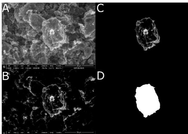
Figure 7. Digital image analysis methodology for target aggregates, (A) original ESEM microphotographs, (b) Image grey level adjustment, (c) target aggregates, (d) measurement the surface area.
