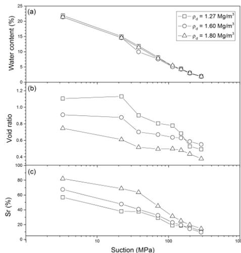
Figure 2. Water content (a), void ratio (b) and degree of saturation (c) versus suction for water retention curve measurements under wetting path at three different dry densities.
