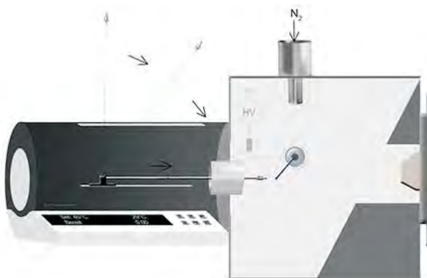
Fig. 1. DART ion source – setup, the helium can be heated up to 500 °C and is excited to metastable state through glow discharge.
