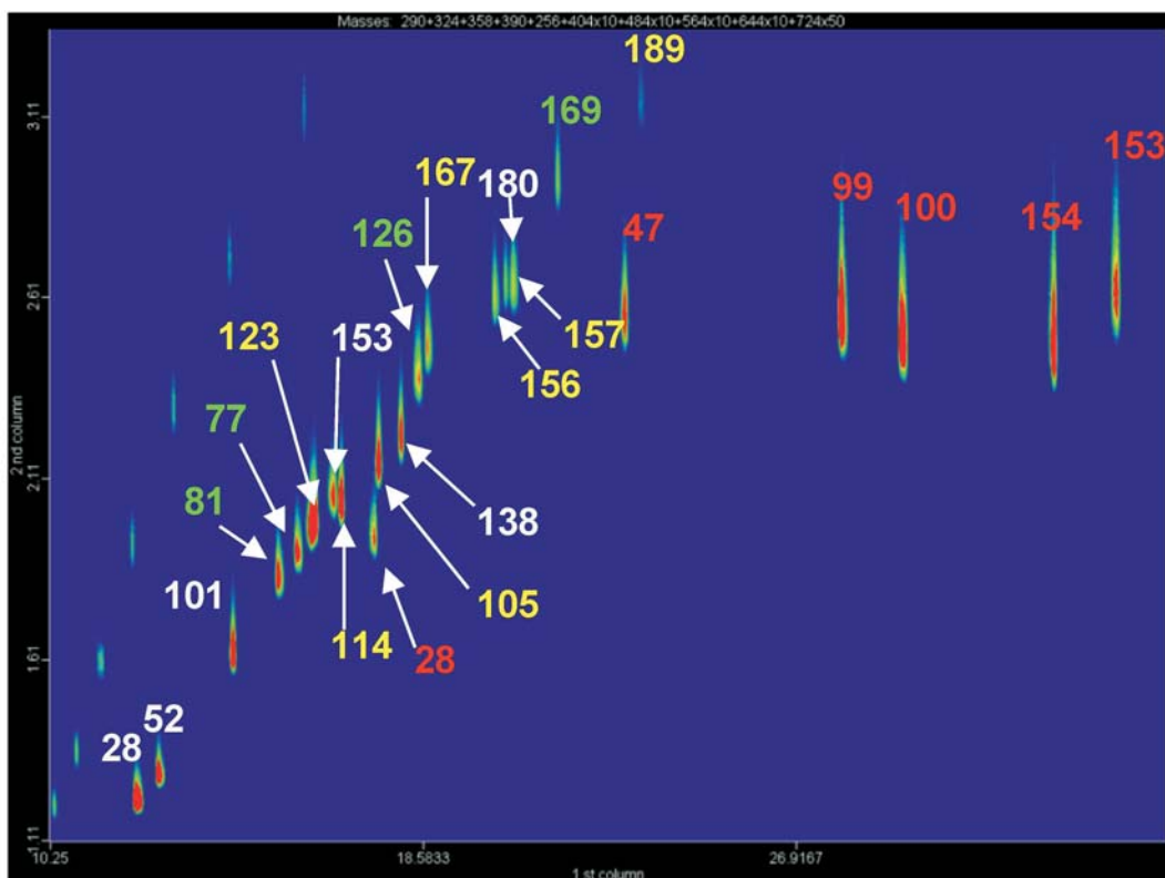
Fig. 1. An example of GC×GC chromatogram of PCBs and PBDEs (200 pg injected) using BPX-50×HT-8 capillary column system; m/z = 256, 290, 324, 358, 390, 404, 484, 564, 644 (yellow mono-ortho PCBs, green non-ortho PCBs, white major PCBs, red PBDEs).
