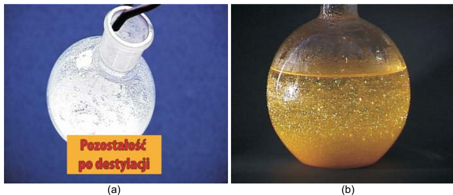
Figure 2. Frames from video presenting interesting chemistry experiments related to certain laboratory techniques e.g. (a) separation of homogenic mixture through distillation, (b) changing the concentration of solutions resulting from crystallization of the diluted substance.
